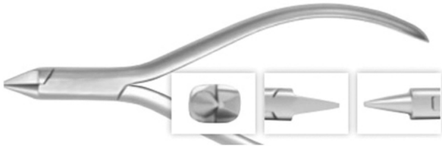
66-5078 Bird Break Plier Plier for working with round wire up to .028" (.71mm). The round beak is precision ground to a perfect cone-.025" at the tip. The pyramid beak is exactly .025" wide at the tips.
