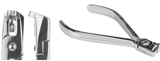
66-5376 Distal End Cutter Flush Cut Safety hold is ideal for cutting wires the patient's mouth. Plier shear-cuts hard wires close to the buccal tube and holds loose wire. Maximum cutting capacity: Archwires up to .022" x .028".
