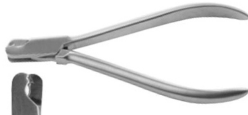
66-5139 Lingual Bar & Facebow Plier Stainless Steel box-joint forging, this instrument is capable of bending wire up to .075" diameter. The plier has large handles and is 3/4" larger than a standard instrument making bending an ease.
