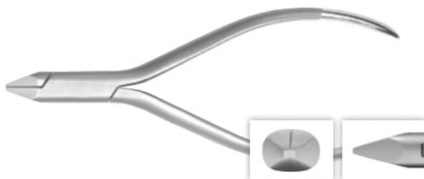
66-5040 Small Adams with T.C. Square beak 1mm at tip and parallel at .045" opening. Effective for wires up to .030" (.76mm)
